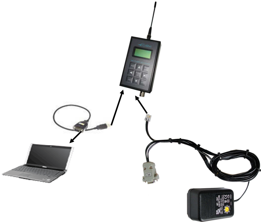
Colibri Flarm, Flarm update configuration
